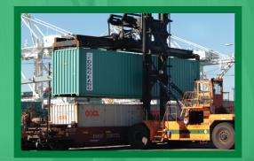
On-dock rail allows goods to transfer directly from ship to a train for direct connection with a distribution network, avoiding extra costly, inefficient movements.
